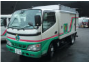
Delivery trucks with additional space for carrying empty bottles and cans to be recycled
