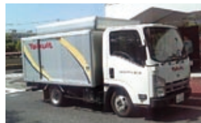
Route delivery truck with a container collection space attached to the roof
