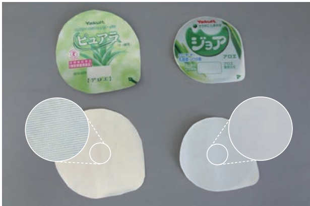
New non-aluminum caps (right) that are more environment-friendly than previously used aluminum caps (left)
