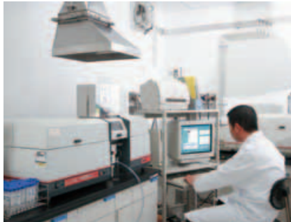
Heavy-metal analysis using an atomic absorption photometer.
