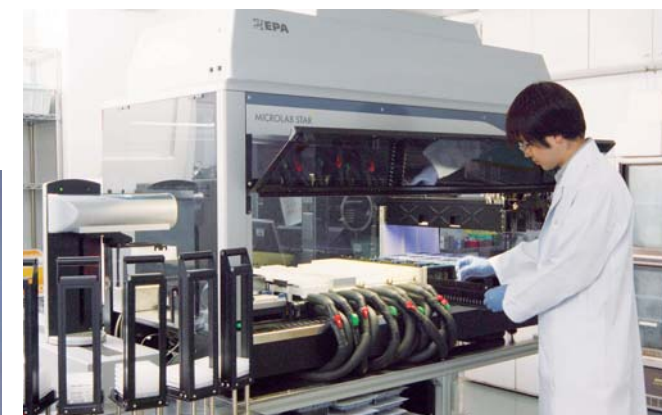
Intestinal Flora Analysis System—"YIF-SCAN" Capable of rapidly analyzing intestinal microflora in a simple, highly precise method without the need for cultivation.
