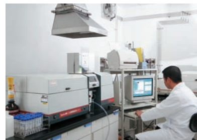
Heavy-metal analysis using an atomic absorption photometer.
