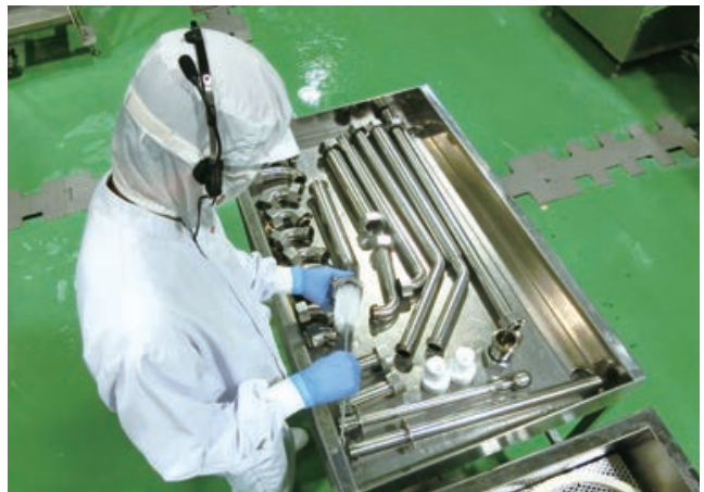
▲Machinery and pipes used in production are disassembled and hand washed every day. We check with our hands and eyes to ensure that everything has been washed and that there are no scratches or other such blemishes. We always clean and disinfect with meticulous care to maintain hygienic conditions.
